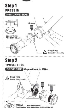
Tool compatible with torque wrench
