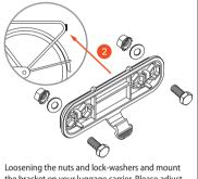
Loosening the nuts and lock-washers and mount the bracket on your luggage carrier. Please adjust the bolts to fit the rear bolt holes, if necessary. Use a wrench firmly mounting the back bracket on your carrier rack.
